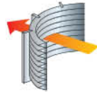
Internal Circumferential Wire Construction
