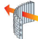
Internal Axial Wire Construction
