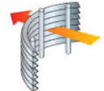
Inverted Wire Construction
