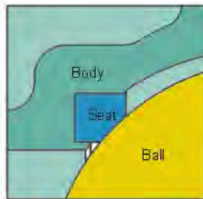
Before Fire Sealing
