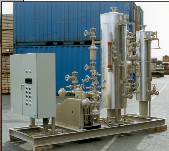
SKID WITH STEAM DRUM
